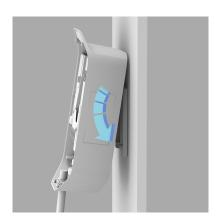
Fasten the charging station on the mounting bracket by tightening the 2x M4 screws.
