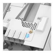
Fasten the copper wire on the corresponding terminal block. The wiring instruction is printed in front of the terminal block (L1/L2/G).
